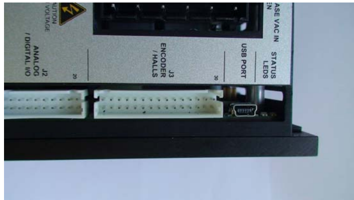
Figure 8: USB Connector / Status LEDs / J2 and J3 Connectors
